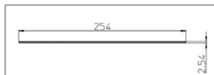
Figure 3. The AA6063 alloy extruded profile under investigation (values in millimeters). Such a thin and wide profile in regards to die diameter is the type of profile that is the most subject to die thermal deformation and cap dishing/deflection.
