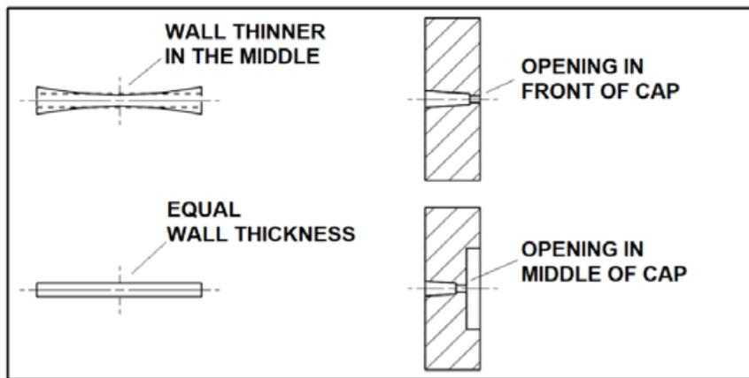
Figure 6. Rendering of the effect of different positions of the bearings in the middle of the cap in terms of wall thickness variation.
