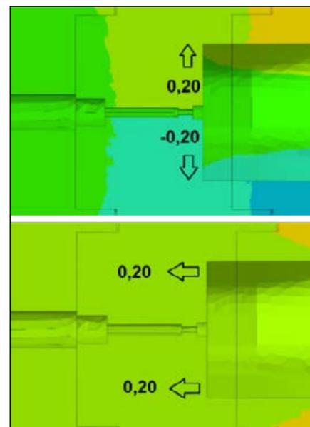
Figure 7. Cap dishing (top) and cap deflection (bottom) at the bearings region of the center of the profile for the novel Design B (values in millimeters). Dishing towards the center and deflection in the extrusion direction look inhibited and minimized respectively.
