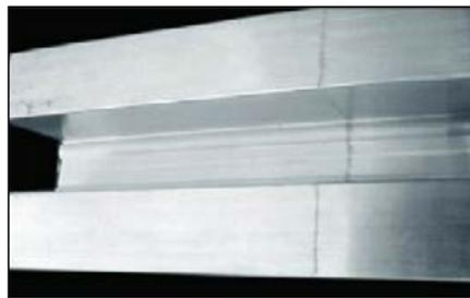
Figure 2. Snap marks on extruded aluminum profile shown at right angle to extrusion direction.
