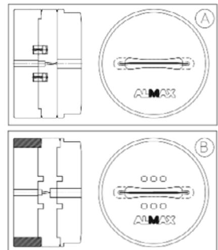
Figure 4. Die designs under investigation showing the front view and vertical cutaway-section. Design A is the benchmark, while Design B is the novel design considered after obtaining the results for the first design.
