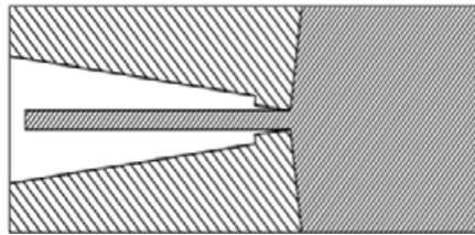
Figure 1. Rendering of cap deformation as a combination of dishing and deflection. Extrusion direction is toward the left.
