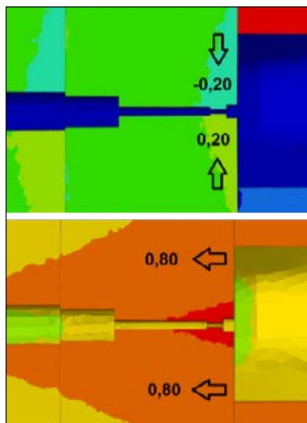
Figure 5 Cap dishing (top) and tool deflection (bottom) at the bearings region in the center of the profile for Design A (values in millimeters). Under load, the deformation of the cap for Design A might generate snap marks.
